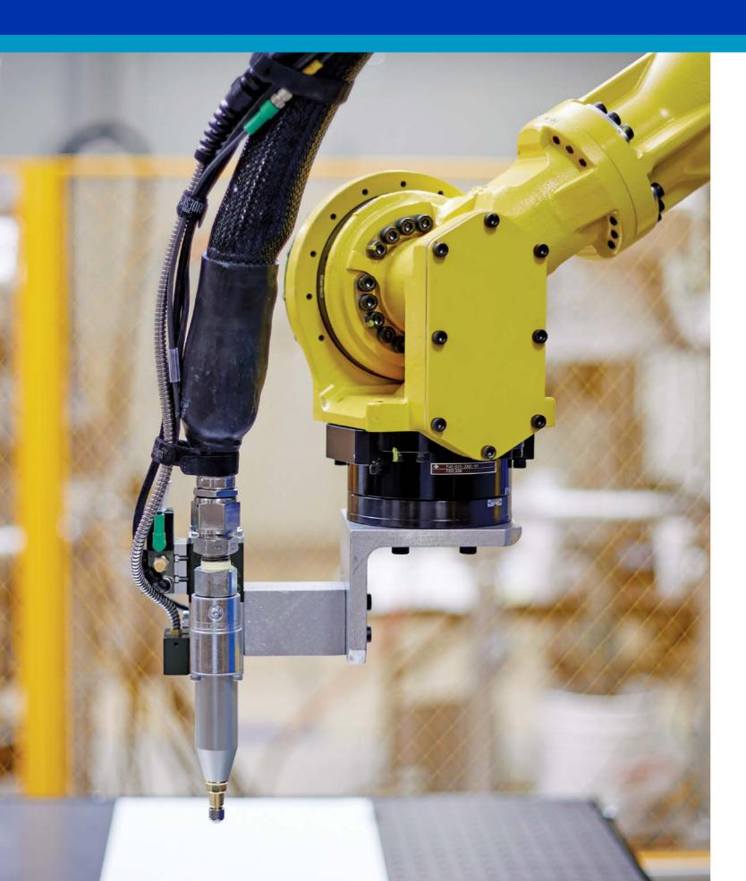
A dispense valve is a critical component in a dispense application because it is the final step of the material handling process. The iQ Dispense Valves were designed with configurable components to meet your application requirements and deliver results you expect.
